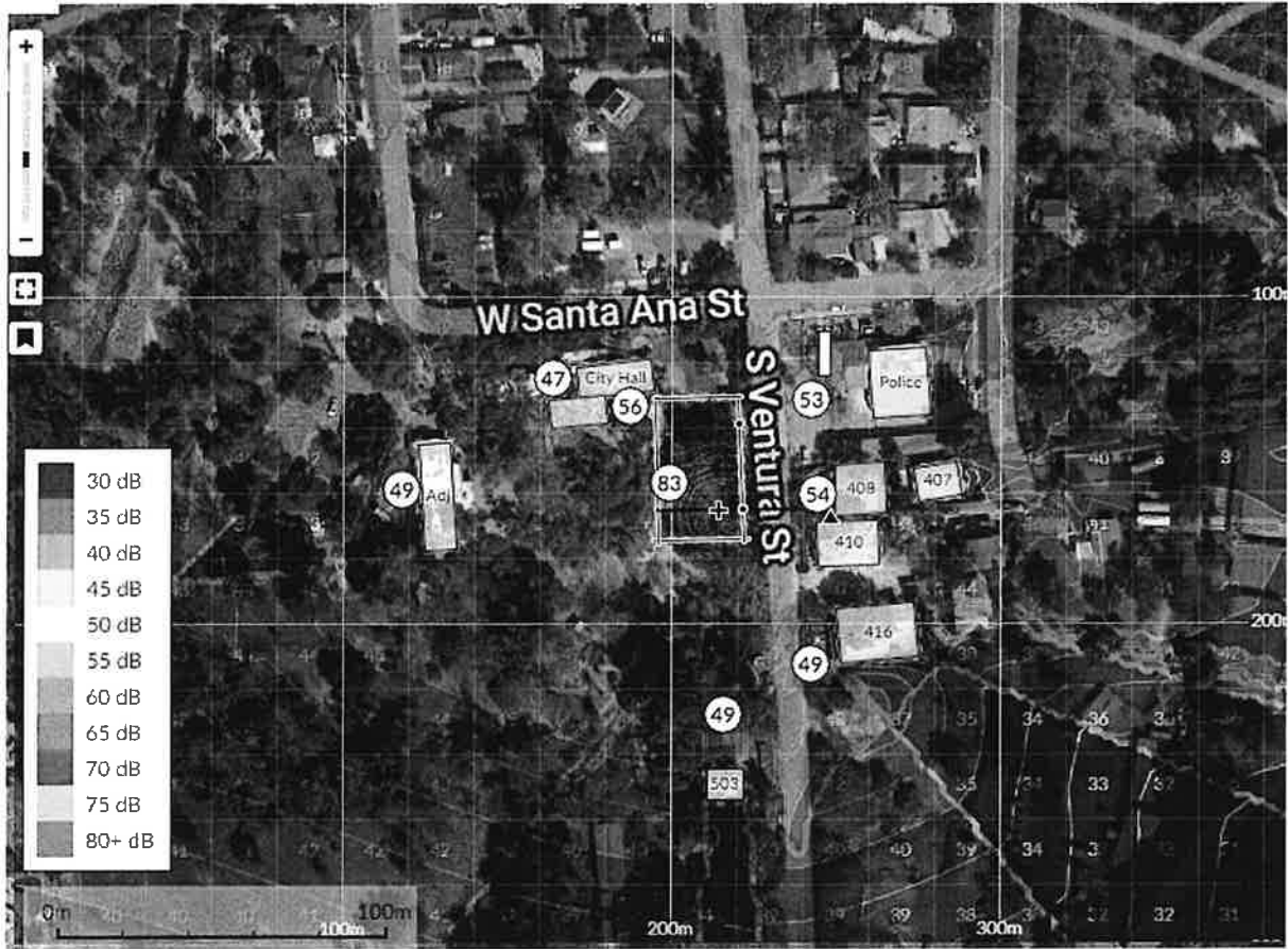
Figure 25 – Plan view showing ray path to South Ventura Street, 30 foot barriers (1 meter = 3.3 feet)
