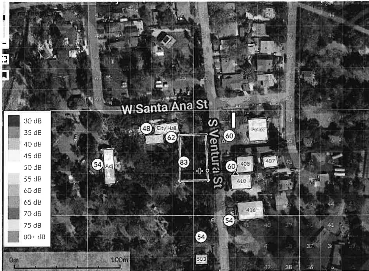
Figure 27 – Plan view showing ray path to South Ventura Street, 15 foot barriers (1 meter= 3.3 feet)
