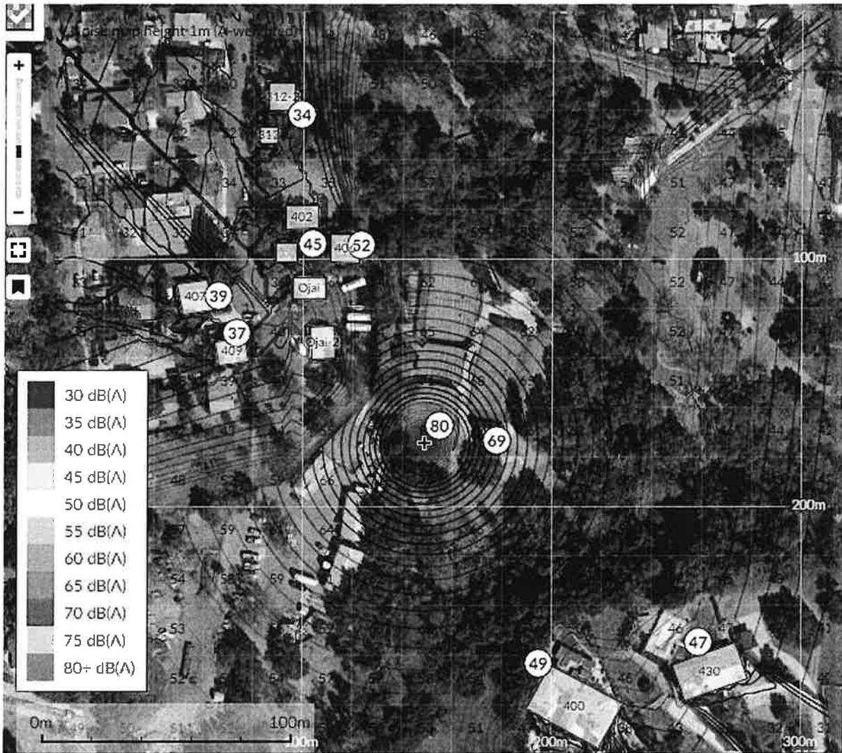
Figure 13 – Noise map for Lower Libbey pickleball courts with dBA lines (1 meter = 3.3 feet)
