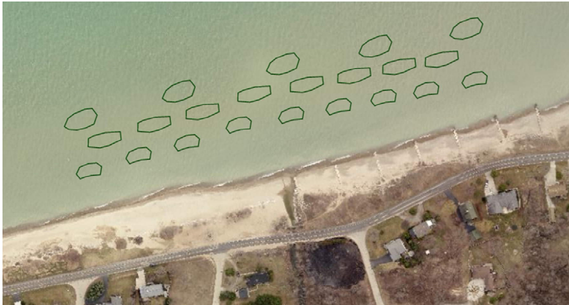
Figure 35: Layout of Offshore Breakwaters
