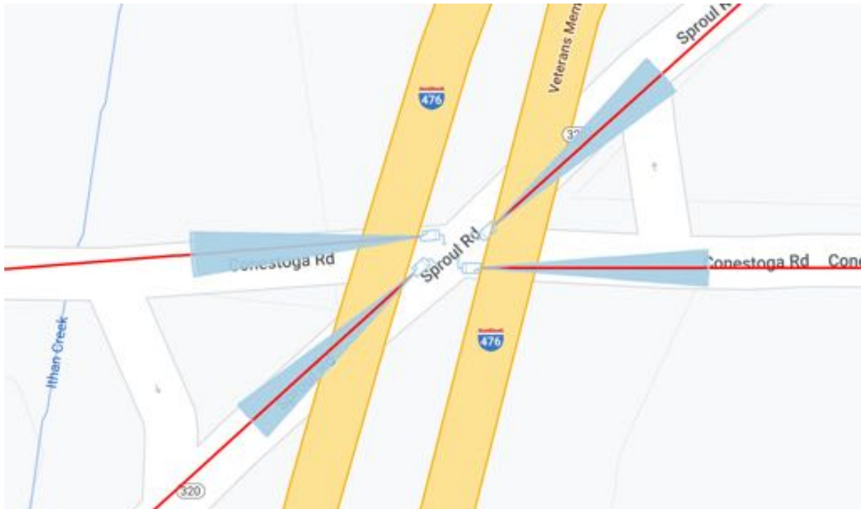
Figure 10 – Rt. 320 / Conestoga Rd. – LPR Overview
