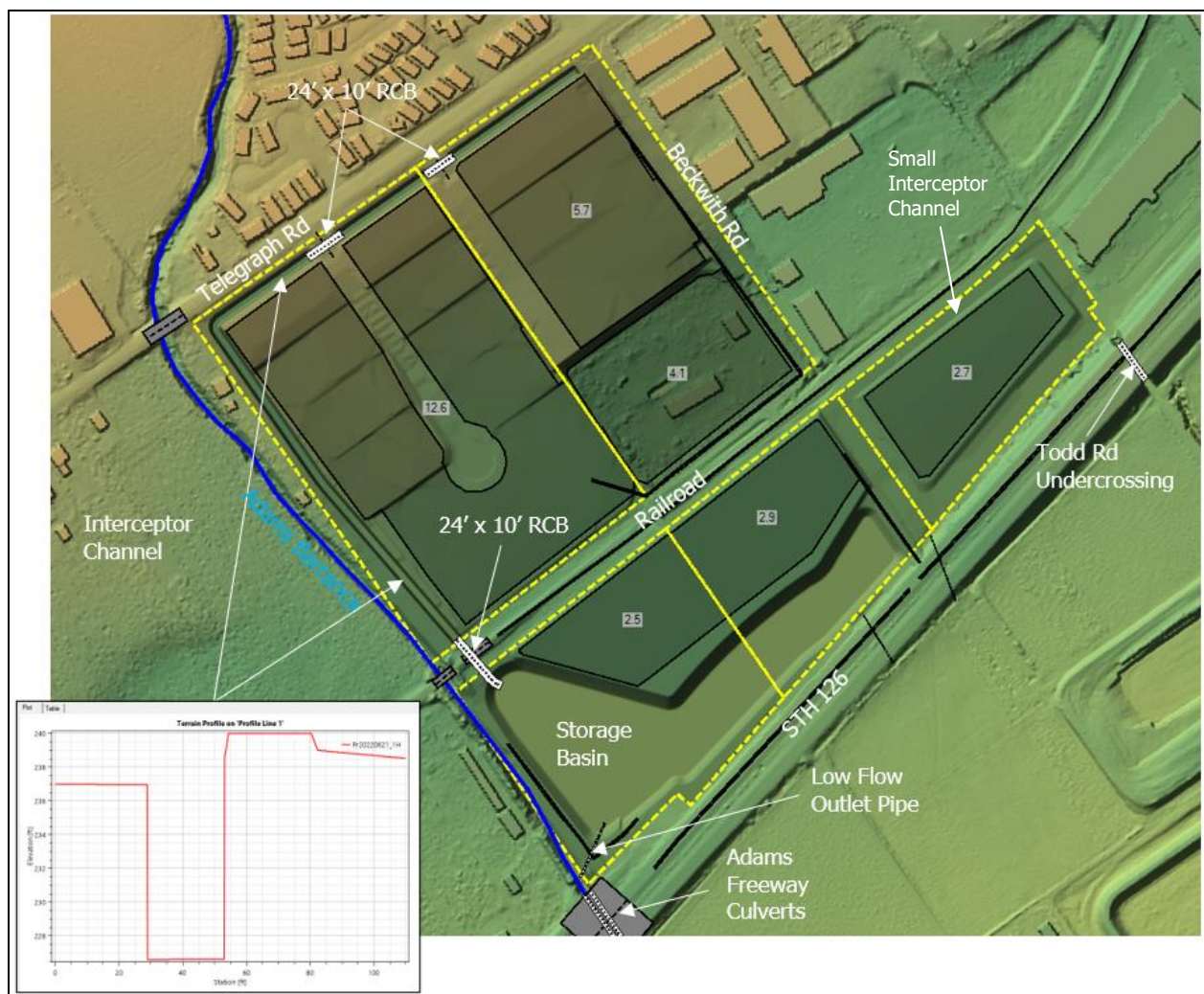
Figure 12: Main Flood Protection Concept Components
