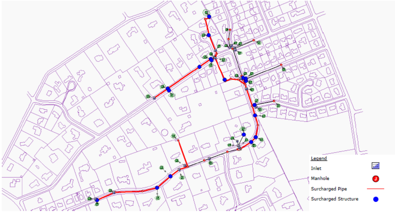
2 Year Storm Plan Plot Cushman Road, Garden Road, Willow Lane & Sheldrake Road
