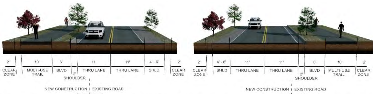
VICTORIA STREET WEST SIDE CONCEPT, TYPICAL SECTION D - D VICTORIA STREET EAST SIDE CONCEPT, TYPICAL SECTION D - D
