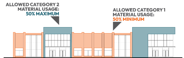
General Commercial (100,000 sq ft or More) Principal Front and Street Side Façade
