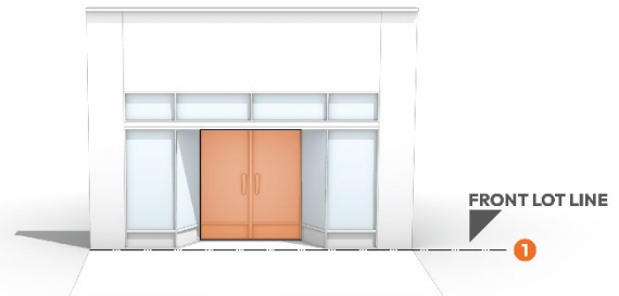
Figure 9: Building Entryway Design - Recessed Entrance
