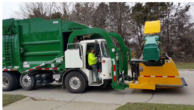
A WM truck equipped with the Auto-Can automated system.
